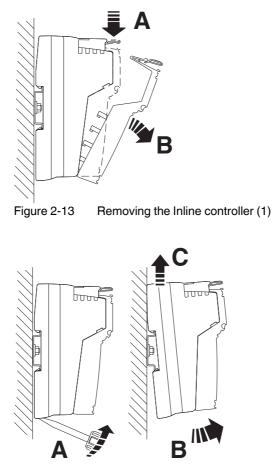
Figure 2-14 Removing the Inline controller (2)
