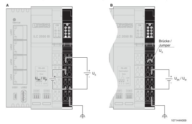
Figure 2-15 shows the basic circuit diagram for the connection of supply voltages.
