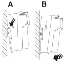
Figure 2-10 Mounting the Inline controller (1)
