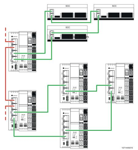
Figure 3-12 Example of Ethernet cabling
