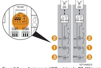
Figure 2-2 Assignment of DIP switches for RS-485 termination
