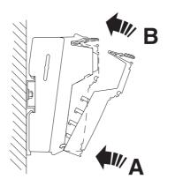
Figure 2-11 Mounting the Inline controller (2)
