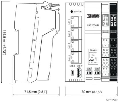
Figure 2-9 Inline controller dimensions
