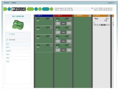
Figure 3-11 Data point test via the startup website
